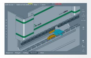
TMM - RA: Advanced CNC controls that power ProBend press brakes can also be Clients of the Praxis Network, communicating in real time the current status of the ongoing process. It is possible to query tool inventory and the current tool set up to optimize bend process for minimum tool changes.
